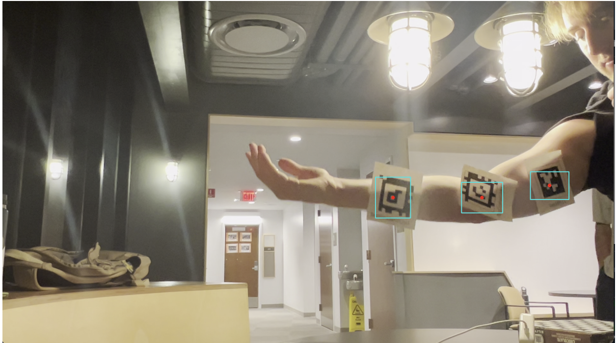
Figure 2 (a): Three points of interest in red being tracked by left camera
